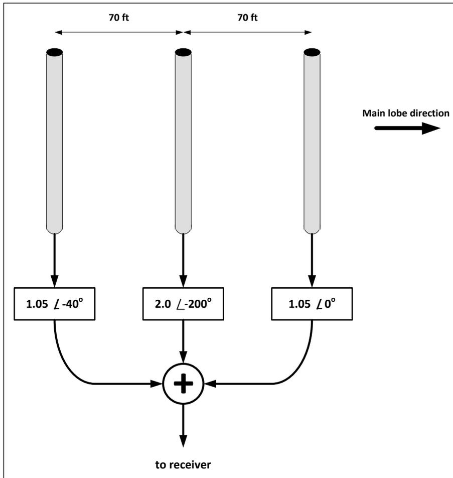
Figure 2 — “Optimized” 3 element inline array for 160 meters
