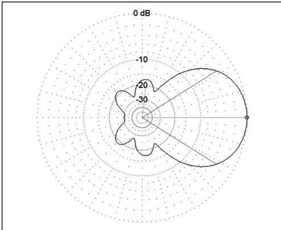
Figure 8 — Azimuth pattern of 800 foot Beverage on 160 meters
