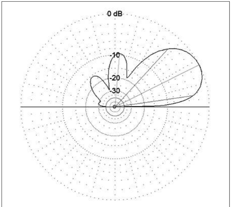
Figure 7 — Elevation pattern of 800 foot Beverage on 160 meters (Note the high-angle secondary lobes.)
