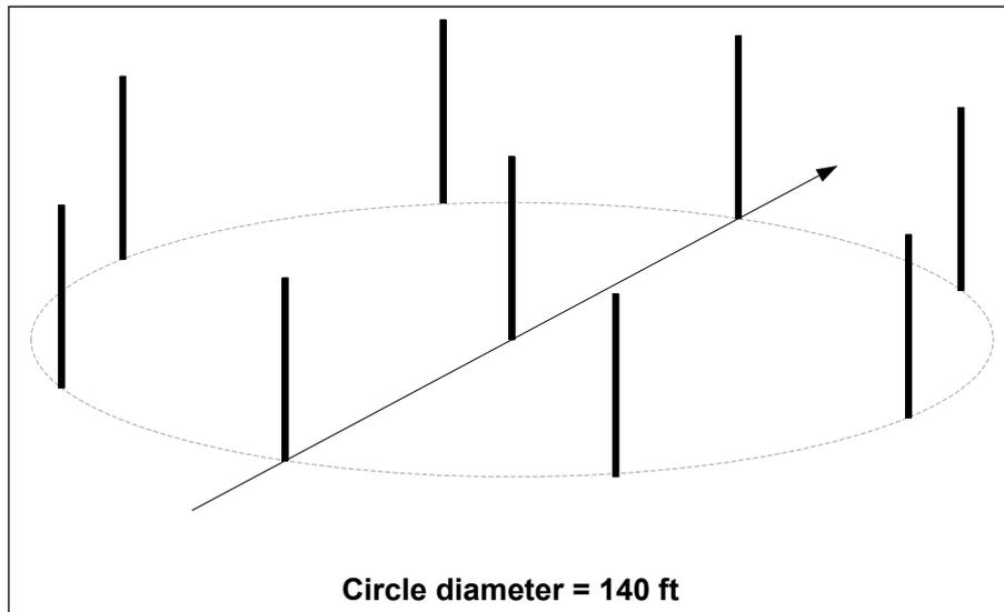
Figure 1 — Nine circle array geometry
