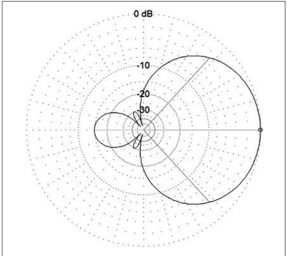
Figure 6 — 80 meter azimuth pattern at a 20° take-off angle.
