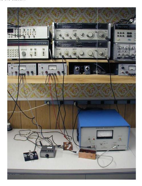
Left to right on the lower portion of the picture: key, keyer, buffer between keyer and signal generator to shape the rise and fall times of the keying, ENI 1040L power amplifier. On the shelf above the amplifier is the HP 8640B signal generator which is keyed via it's modulation input to drive the amplifier. Keyer can be used in the normal mode or in a beacon mode.
