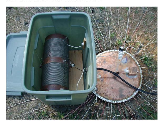
The tuner is just a 90 uH coil in series with the base of the antenna. One end of the coil is grounded and the other end connects to the antenna. Matching is accomplished by tapping up on the coil about three turns from the bottom. The coil is salvage from a BC transmitter and I'm only using the upper half of the coil.
